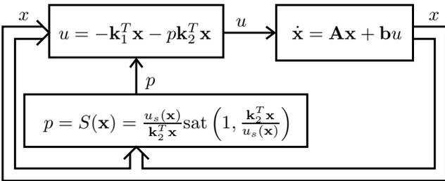
Fig. 11. Structure of the reformulated VSC.
