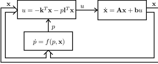
Fig. 7. Structure of the control system conforming to dynamic soft VSC.
