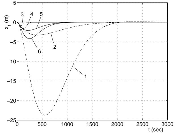
Fig. 14. Dive depth,  $x_1$ , as a function of time,  $t$ . Regulation from the initial state  $\mathbf{x}^T = [0 \ 0 \ -0.0008]$  to the equilibrium state  $\mathbf{x}^T = \mathbf{0}$  using linear control (1), saturated linear control (2), time-optimal control (3), soft VSC employing implicit Lyapunov functions (4), dynamic soft VSC (5), soft VSC with variable saturation (6).
