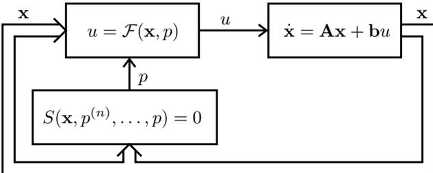
Fig. 2. Block schematic of soft variable structure controls.
