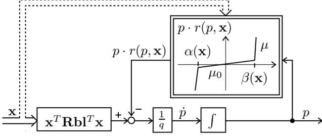
Fig. 9. Block schematic of the differential equation,  $\dot{p} = f(p, \mathbf{x})$ , representing an anti-windup system.
