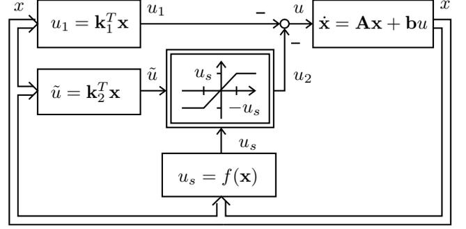
Fig. 10. Structure of the VSC with variable saturation.
