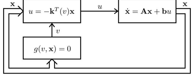
Fig. 4. Structure of the control loop employing an implicitly defined Lyapunov function  $v$  as selection strategy.
