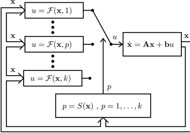
Fig. 1. Block schematic of a discontinuous variable-structure control.
