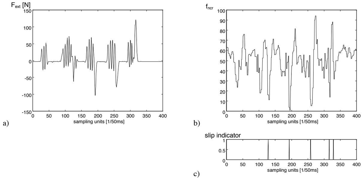
**Fig. 4** The diagrams show the detection of slip due to collisions of the object. Fig. 4a) shows the external force to the object measured by the force/torque sensor and fig. 4b) its influence to the resulting normal force measured by the TMS. In fig. 4c) the results of slip detection is shown, slip is detected if slip detector = 1.
