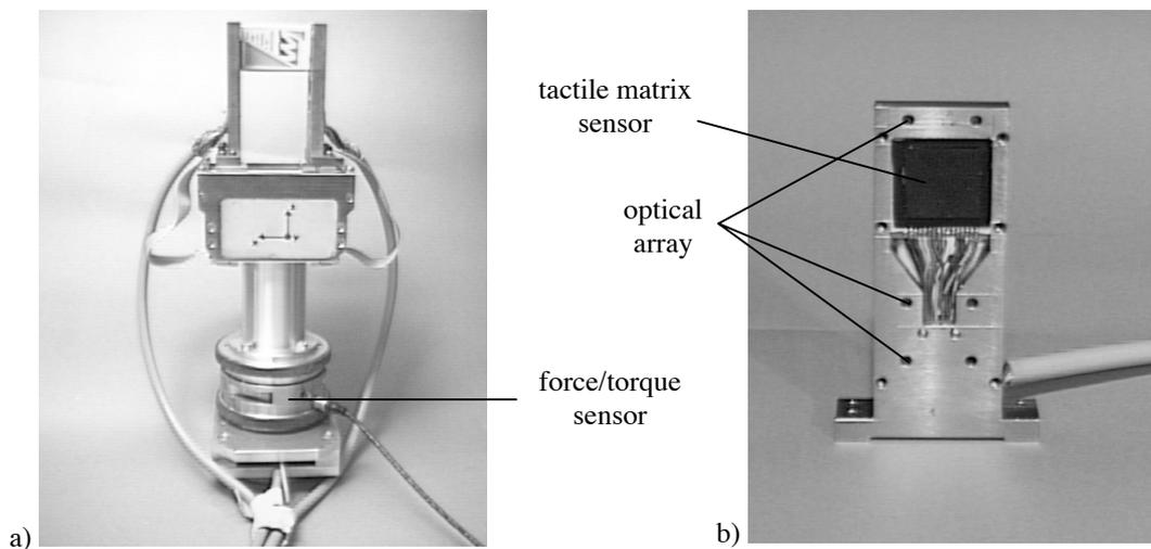
**Fig. 1** The multisensory gripper system. On the left the whole gripper system is shown, grasping a match box. On the right a single gripper jaw with its optical array and the tactile matrix sensor is shown.
