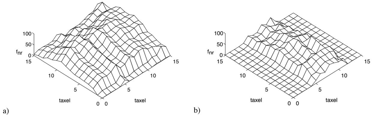
**Fig. 2** This Figure shows two tactile images of the TMS, where a relative force distribution over the sensor surface of 16×16 taxels is illustrated. Fig. 2a) shows a contact to a rather flat object surface, while the contact situation in fig. 2b) is typical for either a cylindrical object or an object grasped at a ledge.
