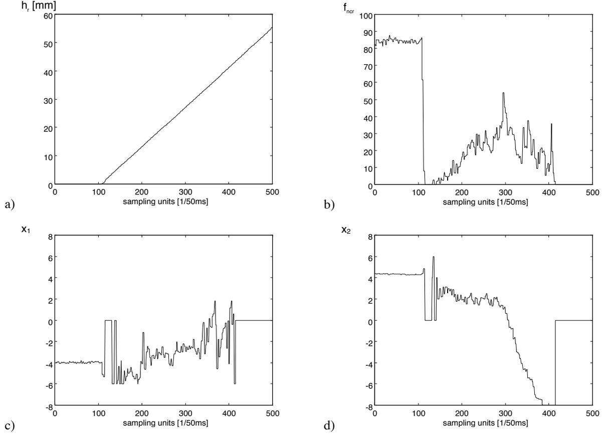
**Fig. 3** The diagrams illustrate the measurements in an artificial experiment with a fixed object slipping out of the moving gripper. In fig. 3a) the movement is shown, while fig. 3b) shows the resulting normal force measured by the TMS of one gripper jaw and fig. 3c) and 3d) illustrate the center point of the force distribution in taxel coordinates.
