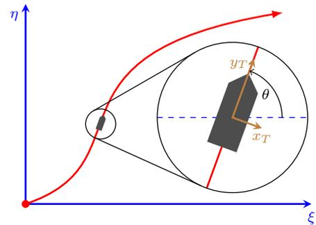
Fig. 4. Definition of the navigation coordinate system (blue) and the train coordinate system (brown).  $\theta$  is the train's orientation angle, measured between the  $\xi$ -axis and the velocity vector in along-track direction. The track is shown in red. The dot marks the track's starting point ( $l = 0$ ) and the arrow the direction of positive counting.
