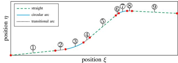
Fig. 1. Exemplary track, consisting of the three standard track geometries: straight, transitional arc and circular arc. The individual parameters for the track elements 1 – 9 are listed in Tab. I.
